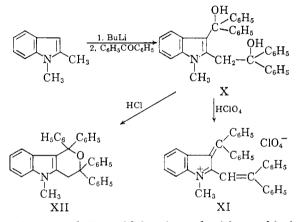
Compound X could be titrated with perchloric acid in acetic acid giving rise to a deep red solution most likely due to structure XI.
